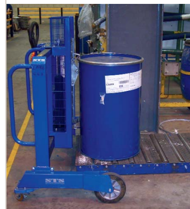
Loading the drum onto the roller bed
